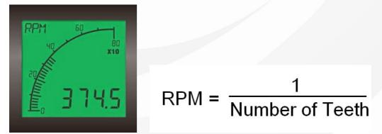
You must first calculate one over the number of pulses from the wheel in one revolution this figure must then be entered into the display scalar section of the APM Configurator software
