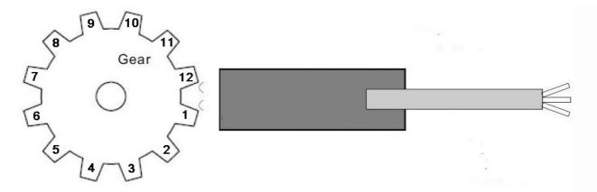
Therefore the scale required is  $1 \div 12 = 0.083$  this is then entered into the scale box which will then mean the scale on the APM can read true RPM
